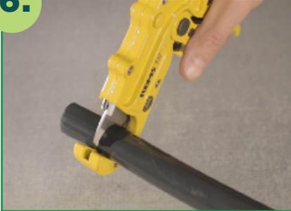
Using a blade-style pipe cutter, make a square cut, being careful to minimize pipe distortion. Manually remove any burrs or debris from pipe end if present.
